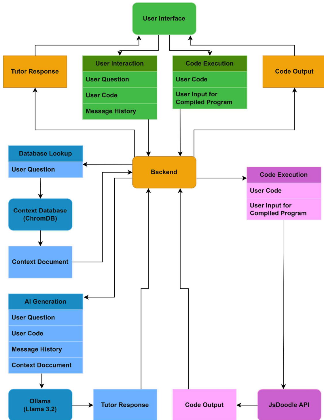
Figure 2 – The Chart above illustrates the flow of information through the application. The green represents the front-end, while the orange is the back-end. The blue represents the answer generation process and the pink represents the code compilation and execution process.
